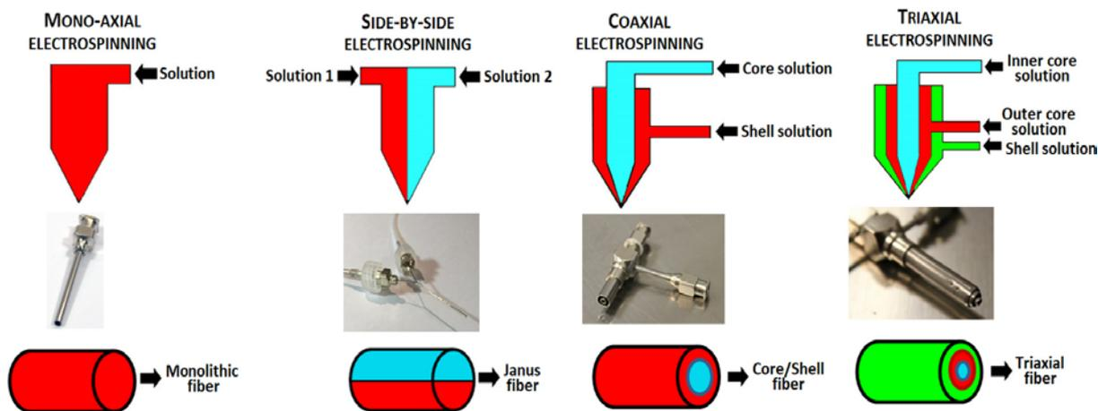
Figure 4. Nozzle configurations [9]
