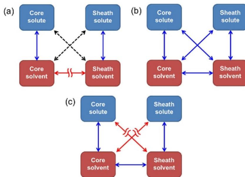
**Figure 3.** Miscibility of core and sheath solutions used in co-axial electrospinning: (a) totally immiscible solutions (solute and solvent); (b) totally miscible solutions (solute and solvent); (c) partially miscible solutions (solvent-only miscible) [35]
