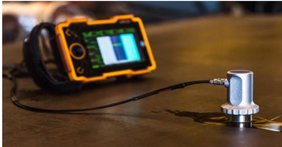
Fig. 8. Ultrasonic testing system
