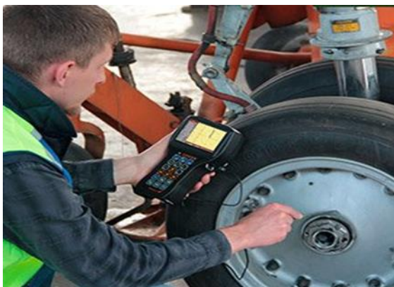
Fig. 6. Eddy current testing of landing gear [20]
