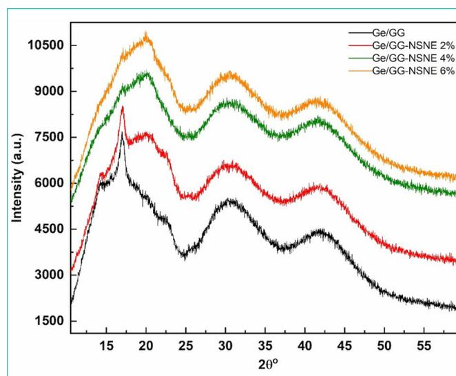
**Figure 1.** XRD diagram of film without NSNE and films loaded with 2% (w/w) NSNE, 4% (w/w) NSNE and 6% (w/w) NSNE
