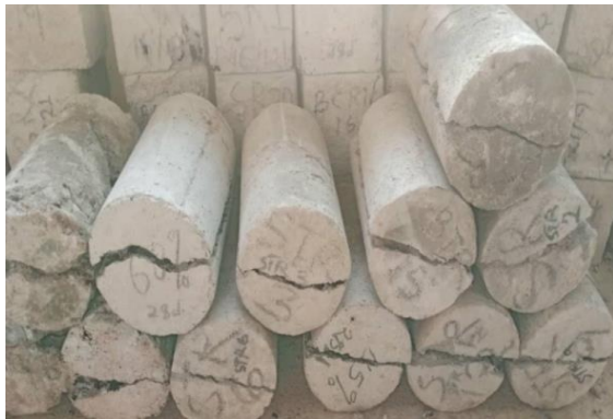
Figure 12a. Crushed Cylindrical samples
