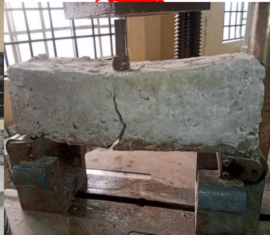
Figure 14b: Beam during testing
