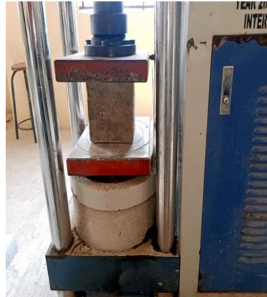
Figure 10b: Cube in testing
