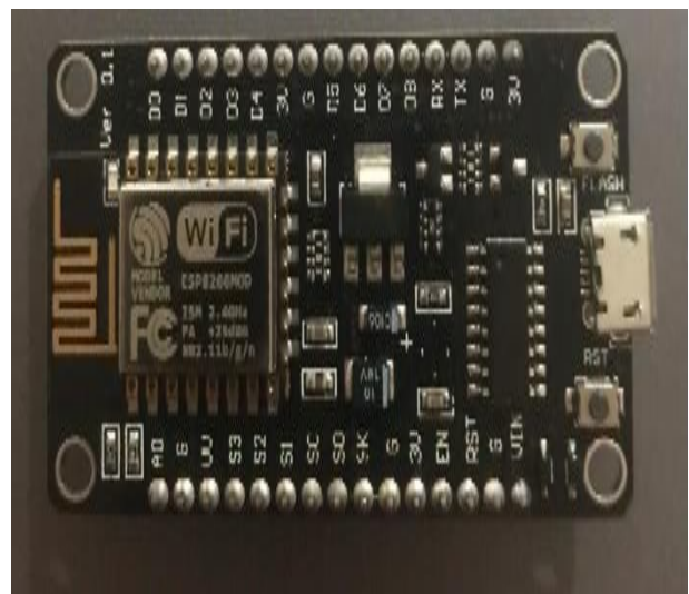
Figure 1. NodeMCU with ESP8266 Wi-Fi module
