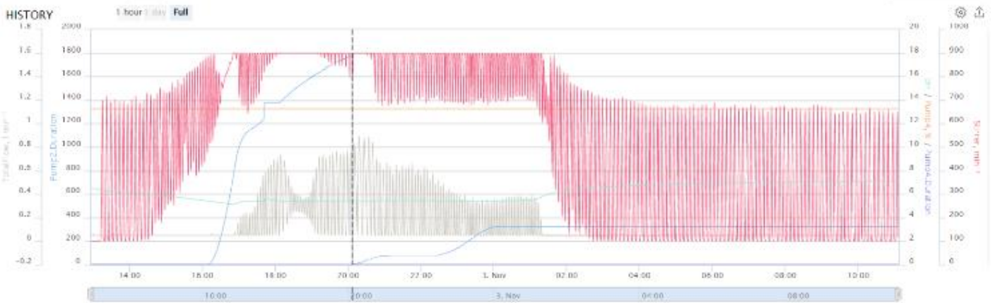
Figure 3. The evolution of pO 2 , pH, agitation, temperature, base pump duration over time. The graph shows the pH level (blue), stirrer (pink), base pump duration (dark blue), total flow (grey).
