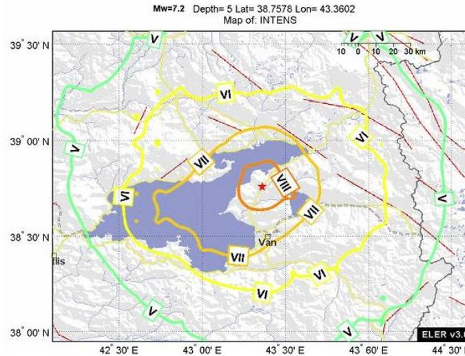
**Fig.2.** Instrumental intensities associated with the main shock (Koeri, 2011)
