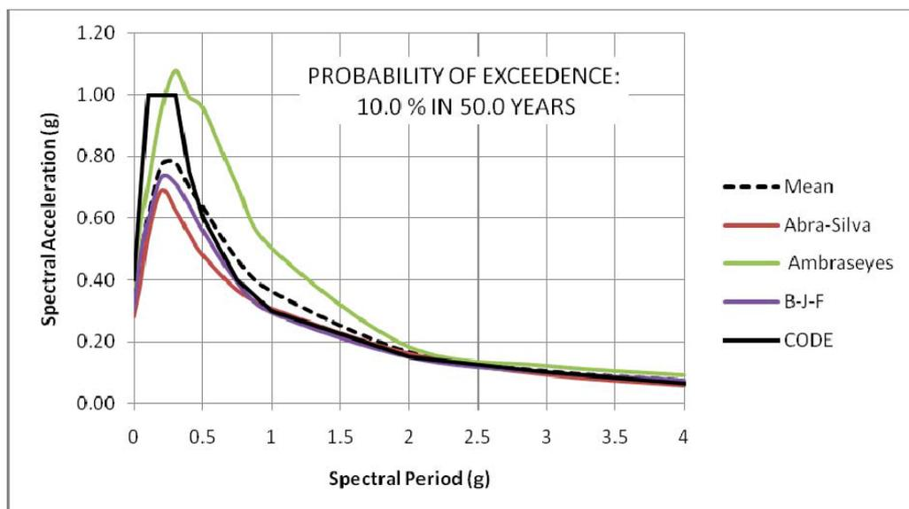
Fig.8. Comparison of spectral responses at 5% damping for the return period of 474.6 years in Bitlis (Kutanis et al. 2010).
