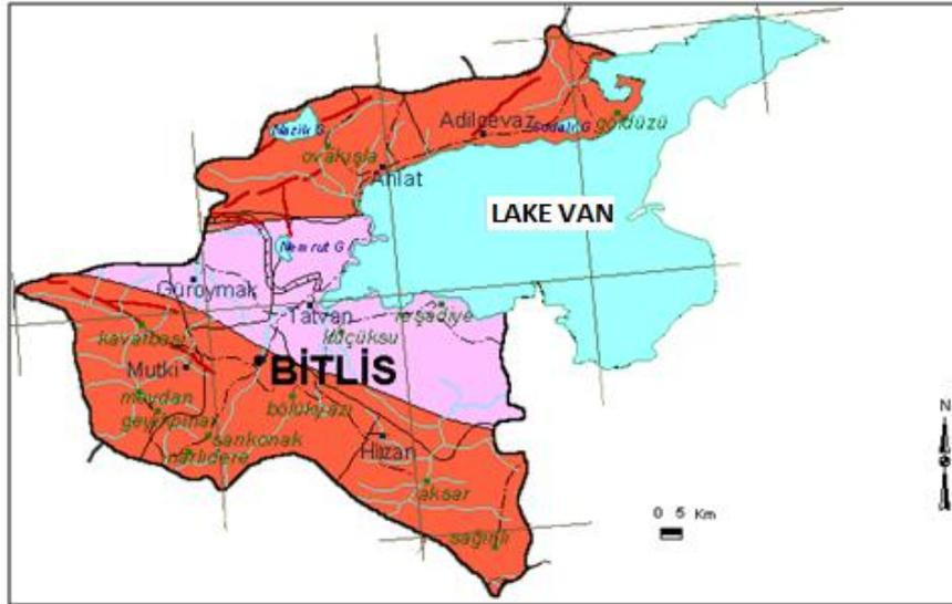
**Fig.6.** Seismic hazard map of Bitlis where the red areas indicate first degree zone with a minimum effective acceleration of 0.40 g and the pink areas for the second degree with 0.30 g
