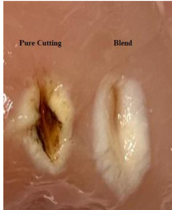
Figure 15. Cutting results on the chicken breast
