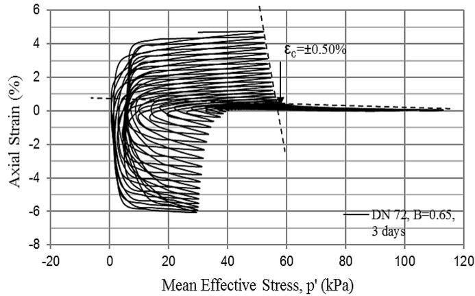
**Figure 12.** DN72, Axial strain – Mean effective Stress.
