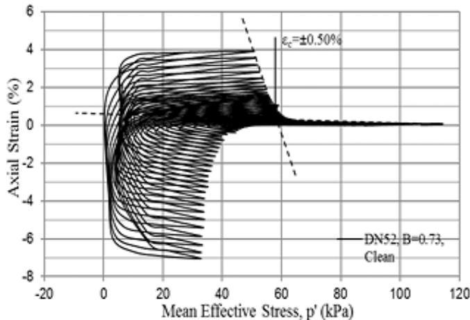
Figure 11. DN52, Axial strain – Mean effective Stress.
