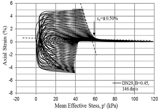
**Figure 13.** DN29, Axial strain – Mean effective Stress.
