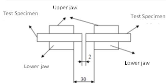
**Figure 2.** Binding of samples to the jaw
