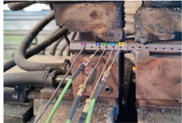
Figure 4. Arrangements of thermocouples on the sample
