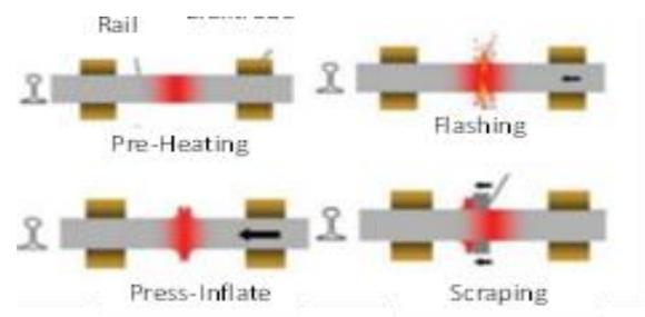
**Figure 3.** Flash butt welding process steps [8]
