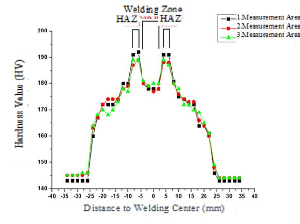
Figure 8. Graph of hardness test results
