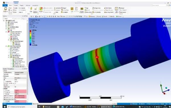
**Figure 15.** Thermal analysis after welding
