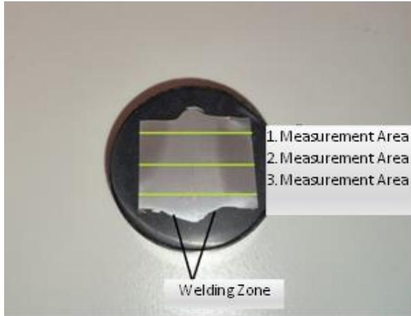
Figure 7. Regions where hardness testing is performed
