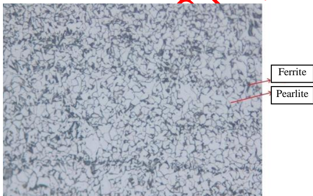
Figure 11. Image of the area under the influence of heat (HAZ)
