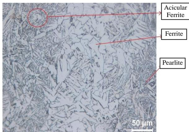
**Figure 12.** Image of the weld metal.
