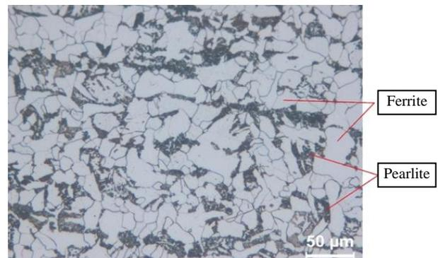
Figure 10. Image of the region that has not undergone heat change (base metal)
