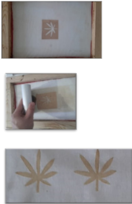
Image 4. Pattern fixed on screen printing sieve/ Screen printing processes/ Printed cotton fabric
