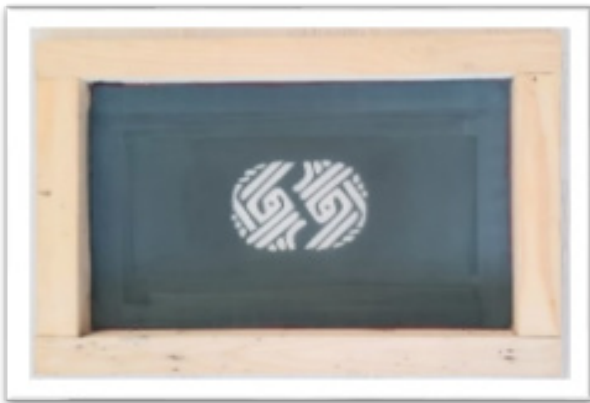
Image 3. The pattern is exposed to the screen printing mold
