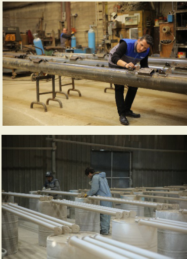
Figure 3. Preparation of S235JR steel construction
