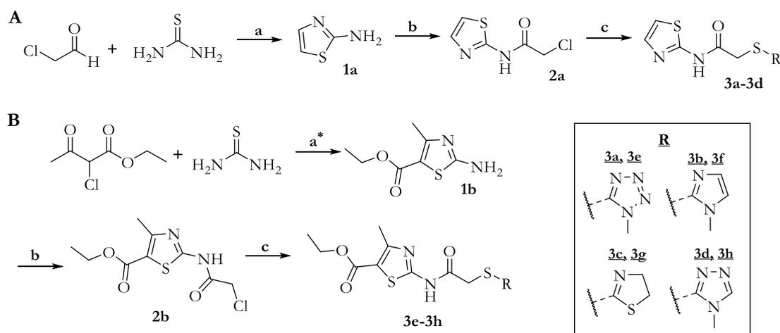
**Scheme 1. Synthesis plan. A: Stepwise synthesis of compounds 3a-3d, B: Stepwise synthesis of compounds 3e-3h; a:** EtOH, reflux 4 hrs; **a\*:** THF, 0°C/rt 30 min/reflux 8 hrs; **b:** 2-chloroacetyl chloride, THF, TEA, 0°C, **c:** Mercaptoheterocycles,  $\text{Me}_2\text{CO}$ ,  $\text{K}_2\text{CO}_3$ , rt. 2 hrs.
