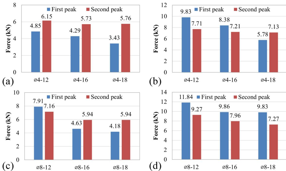
**Figure 5.** Contact forces of sandwich specimens, with Ø4 mm diameter pins tested with (a) Ø12.7 mm and (b) Ø20 mm indenters, with Ø8 mm diameter pins tested with (c) Ø12.7 mm and (d) Ø20 mm indenters
