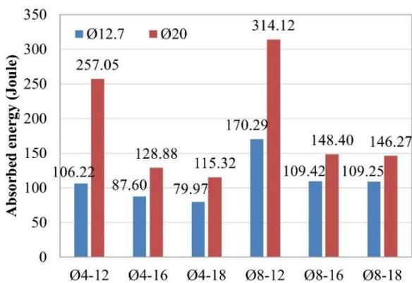
**Figure 6.** Absorbed energy values of sandwich specimens
