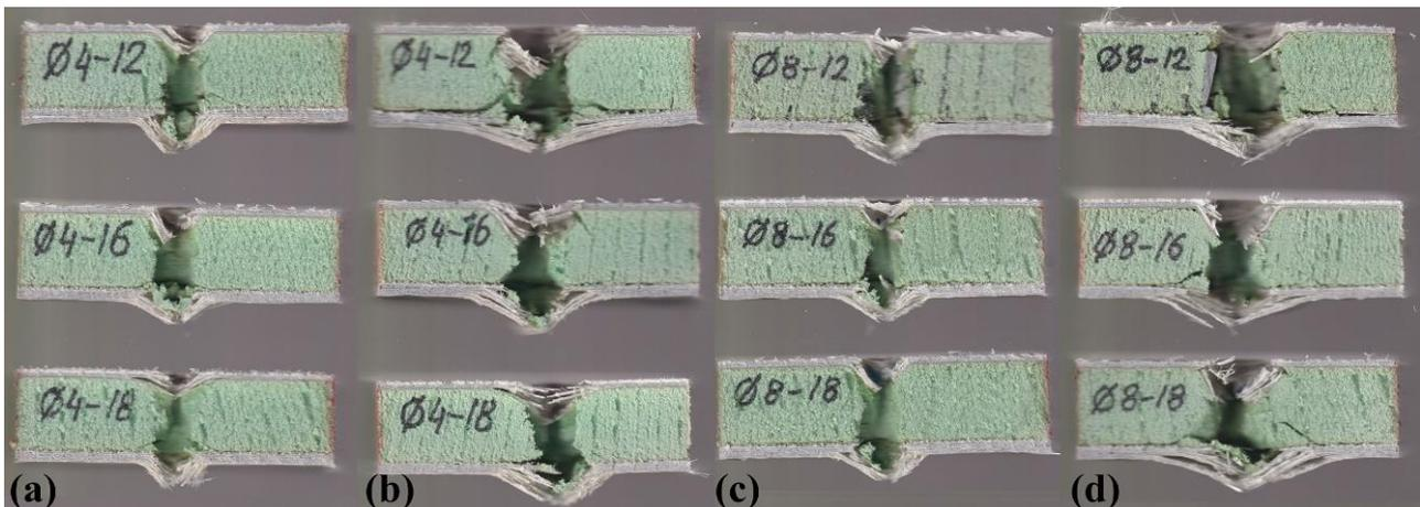
Figure 7. Cross-sectional images of damaged sandwich specimens
