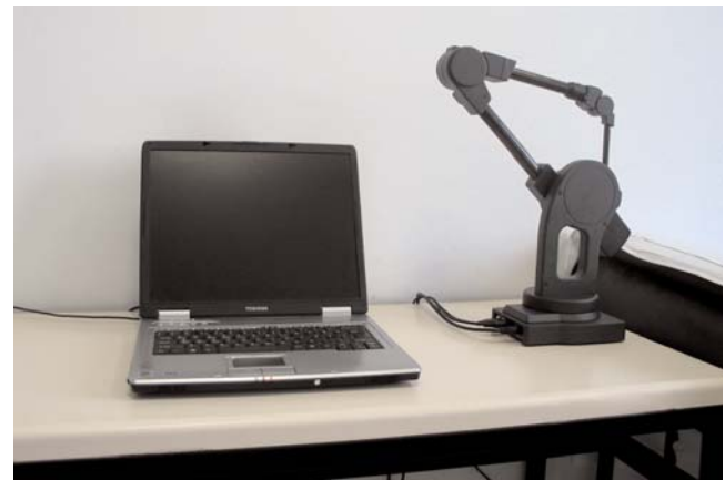
Figure 2. Microscribe digitizing system.
