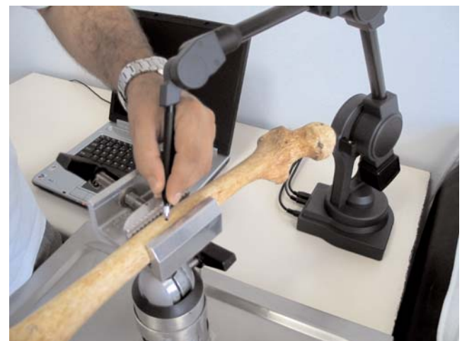
Figure 3. Measurements performed by microscribe digitizing system on femur fixed with clamp.
