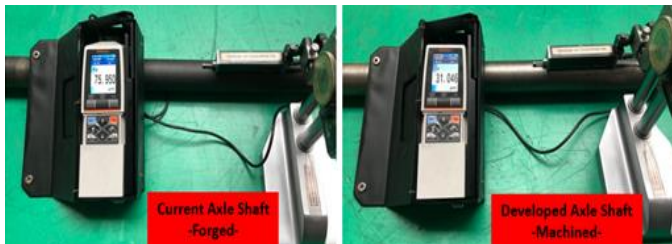
Fig. 6. Comparison of axle shaft surface condition
