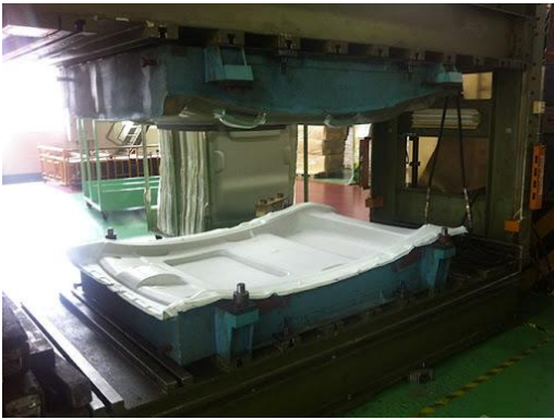
Figure 4. Headliner composite process [8]
