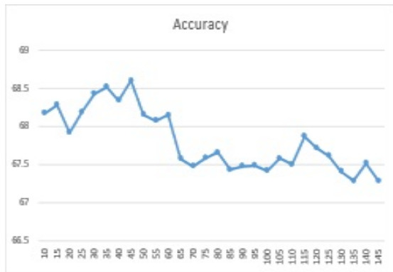
Fig. 10 Accuracy graph for AdaBoost with varying n_estimators.
