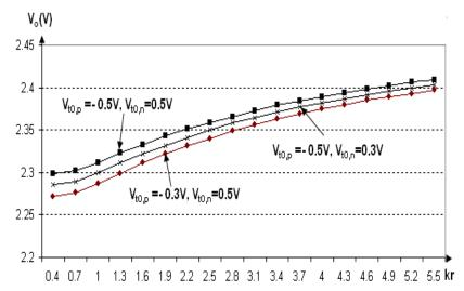
Figure 5. Influence of MOS transistor transconductance parameters ratio  $(k_r)$  on output voltage value  $V_o$ , when the input terminal of CMOS inverter is biased by voltage  $V_{in} = V_{IL}$ , for several parametric values of complementary MOS transistor threshold voltage.
