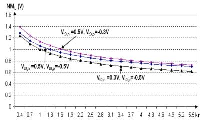
Figure 10. The dependence of the noise margins for low logic level  $NM_L$  on complementary MOS transistors transconductance parameters ratio  $k_r$ , for three cases of different MOS transistor threshold voltage (NMOS and PMOS transistors), when  $V_{DD} = 2.5 \text{ V}$ .
