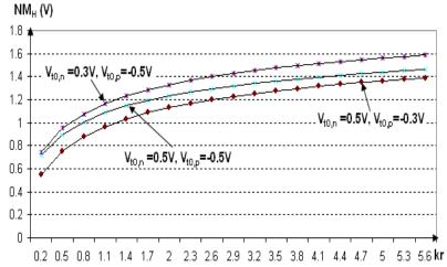
Figure 11. The dependence of the noise margins for high logic level  $NM_H$  on complementary MOS transistors transconductance parameters ratio  $k_r$ , for three cases of different MOS transistor threshold voltage (NMOS and PMOS transistors), when  $V_{DD} = 2.5 \text{ V}$ .
