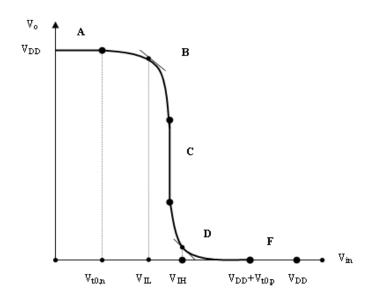
Figure 2. The typical VTC of the CMOS inverter.
