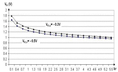
Figure 9. The impact of the transconductance parameters ratio  $(k_r)$  of MOS transistors (NMOS and PMOS) on value of the CMOS inverter threshold voltage  $V_{th}$  (on value of CMOS inverter switching threshold voltage) for two different values of the PMOS threshold voltage, when  $V_{t0,n} = 0.5 \text{ V}$  and  $V_{DD} = 2.5 \text{ V}$ .
