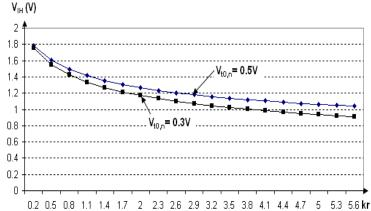
Figure 6. The dependence of the voltage critical value  $V_{IH}$  on MOS transistors transconductance parameters ratio  $k_r$  for two parametric values of NMOS transistor threshold voltage, when PMOS transistor threshold voltage remains constant  $V_{t0,p} = -0.5 \text{ V}$ .
