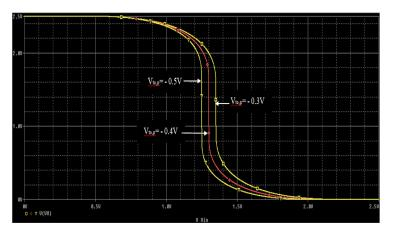
Figure 14. The impact of PMOS transistor threshold voltage ( $V_{t0,p}$ ) on CMOS inverter VTC shape, when NMOS transistor threshold voltage value is  $V_{t0,n} = 0.5$  V, and transistors have identical dimensions.
