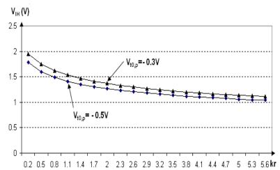
Figure 7. The dependence of voltage critical value  $V_{IH}$  on MOS transistors transconductance parameters ratio  $k_r$  for two parametric values of PMOS transistor threshold voltage, when NMOS transistor threshold voltage remains constant  $V_{t0,n} = 0.5 \text{ V}$ .
