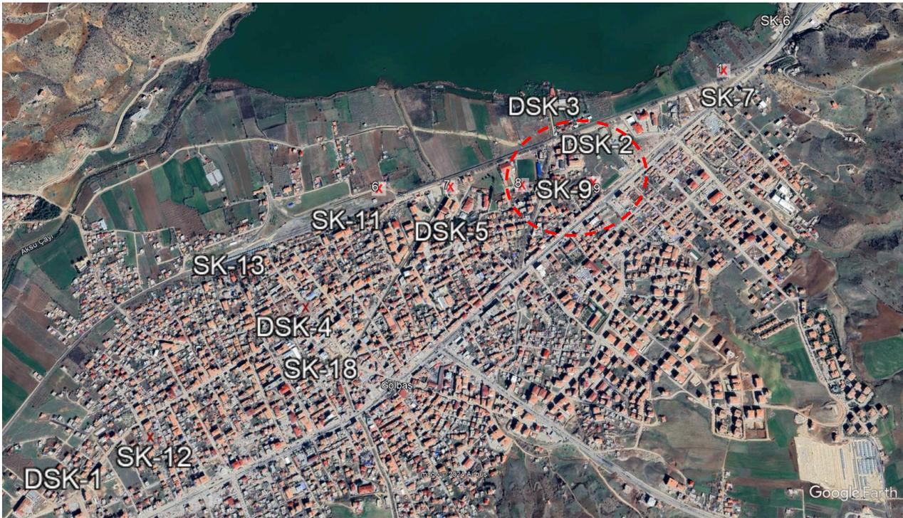
**Figure 7.** Locations of pre and post-earthquake boreholes (SK-x: pre-earthquake; DSK-x: post-earthquake; -x: microtremor).
