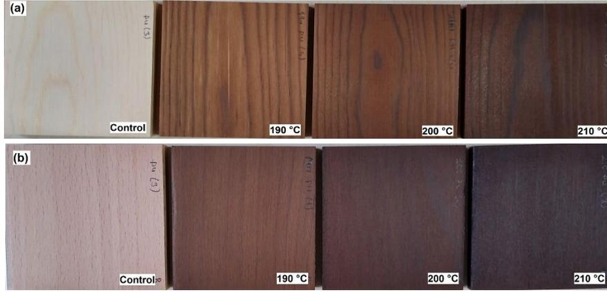
Figure 6. Appearance of scots pine (a) and Eastern beech (b) samples before and after heat treatment
