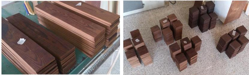
Figure 3. Cutting of samples after heat treatment
