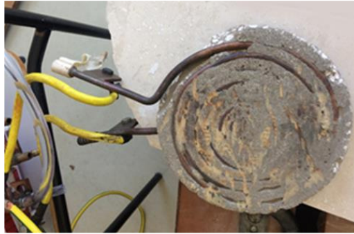
Figure 16. The pancake shaped (spiral) coil used in experimental study
