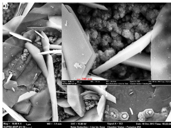
Figure 3a. Relatively low (10000X) and high (50000) magnification top-view SEM images of ZnO films obtained in -0.80 V
