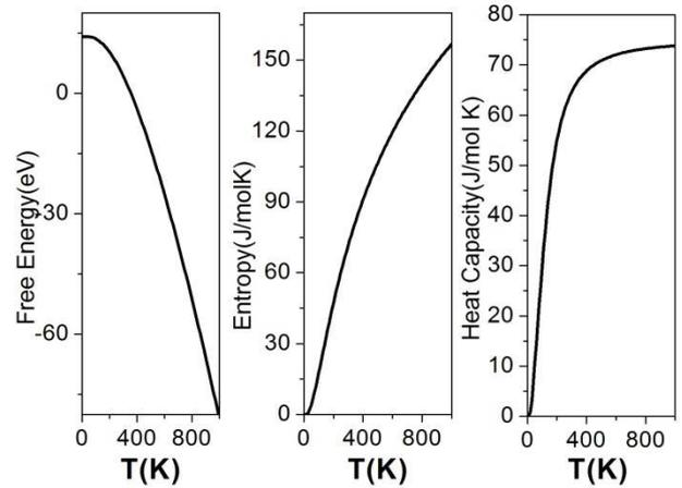
Figure 7. Thermodynamic properties of half-Heusler LiScPb compound
