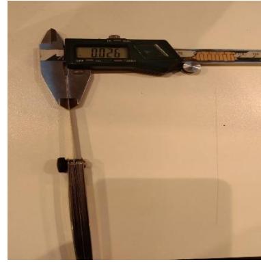
Figure 11. Measurement of bending deflection after the application of 224 J of kinetic energy.
