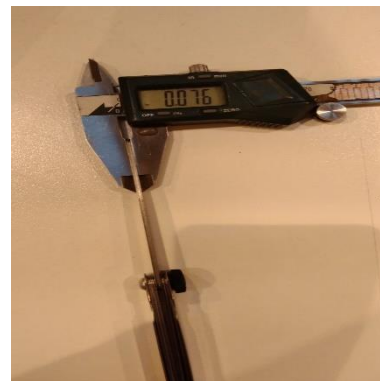
Figure 10. Measurement of bending deflection after the application of 276 J of kinetic energy.
