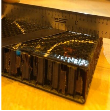
Figure 11. Measurement of bending deflection after the application of 224 J of kinetic energy.
