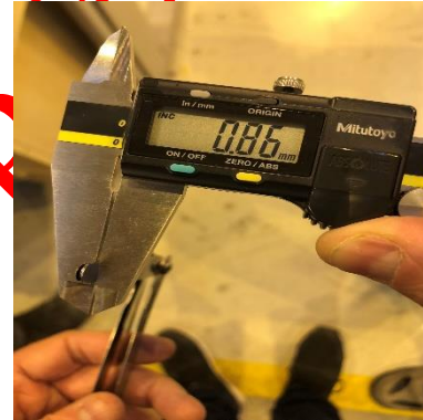
Figure 9. Measurement of bending deflection after the application of 380 J of kinetic energy.
