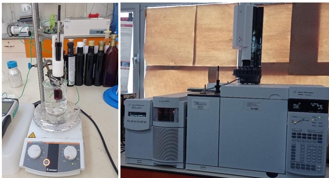
Figure 2. Headspace-solid phase microextraction (HS-SPME) method and GC-MS analysis
