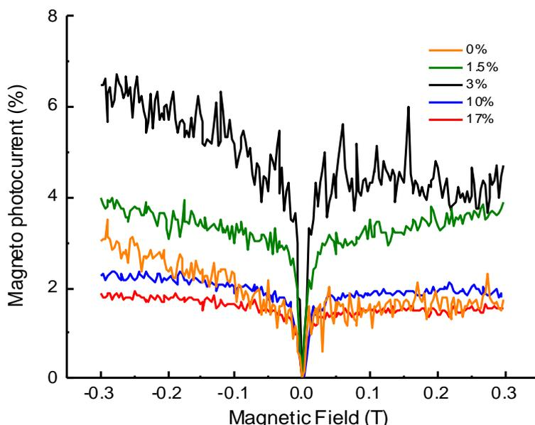
**Figure 4.** MPC response of OPV devices doped with various wt.% of galvinoxyl radical up to field, B of 300 mT.
