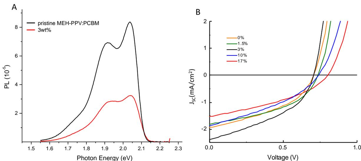
**Figure3.** A) PL spectrum of pristine and galvinoxyl doped (3 wt.%) MEH-PPV:PCBM blend film and OPV device and B)  $I$ - $V$  characteristics of the OPV solar cells doped with various wt.% of galvinoxyl radical.
