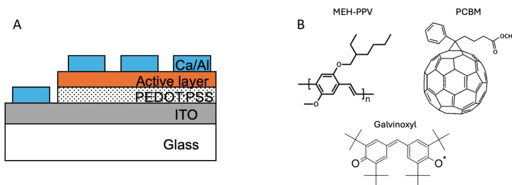
**Figure 1.** A) Device structure of OLED, B) Chemical structures of MEH-PPV, PCBM and galvinoxyl.
