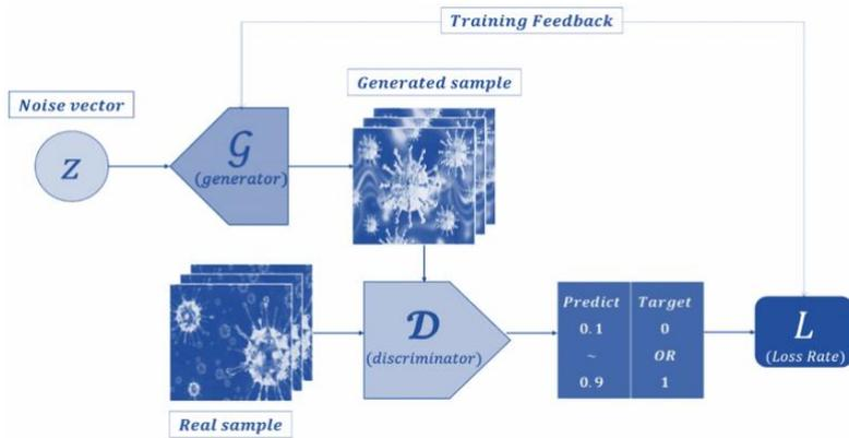
**Figure 3:** Working principle of the GAN algorithm (Park et al., 2021).
