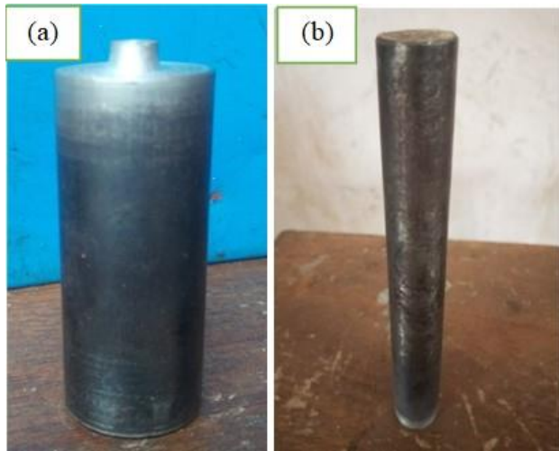
Figure 2. The H13 tool steel used for welding (a) probe tool (b) probe-less tool.
