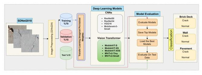
Figure 2. Stages of the proposed crack detection approach
