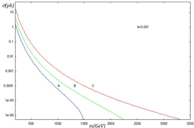
Figure 6. Total cross section for color octet tau leptons versus its mass  $m$  setting to three different machines taking  $k = 0.001$ , curve A with  $\sqrt{s} = 5 \text{ TeV}$ , curve B with  $\sqrt{s} = 10 \text{ TeV}$  and curve C with  $\sqrt{s} = 15 \text{ TeV}$  at  $\tau^+\tau^-$  colliders.
