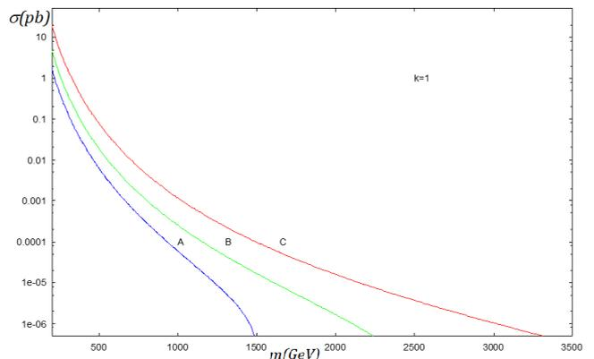
Figure 3. Total cross section for color octet tau leptons versus its mass  $m$  setting to three different machines taking  $k = 1$ , curve A with  $\sqrt{s} = 5 \text{ TeV}$ , curve B with  $\sqrt{s} = 10 \text{ TeV}$  and curve C with  $\sqrt{s} = 15 \text{ TeV}$  at  $\tau^+\tau^-$  colliders.
