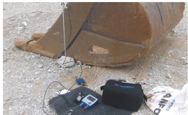
Figure 6. Detection of a monitor station point by GPS
