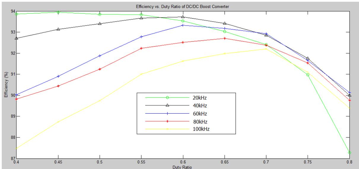
Figure 5. Efficiency vs. duty ratio graph of boost converter with respect to switching frequency
