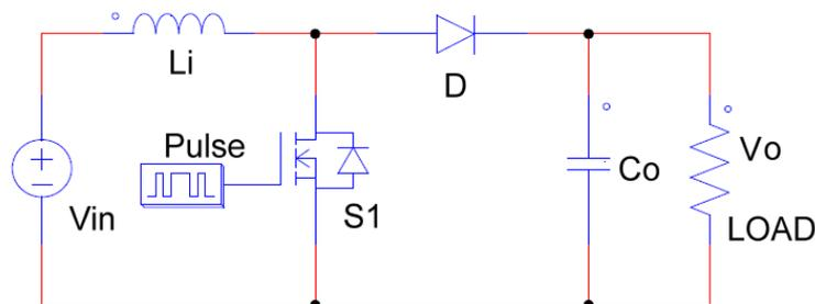
Figure 1. Ideal DC/DC boost converter
