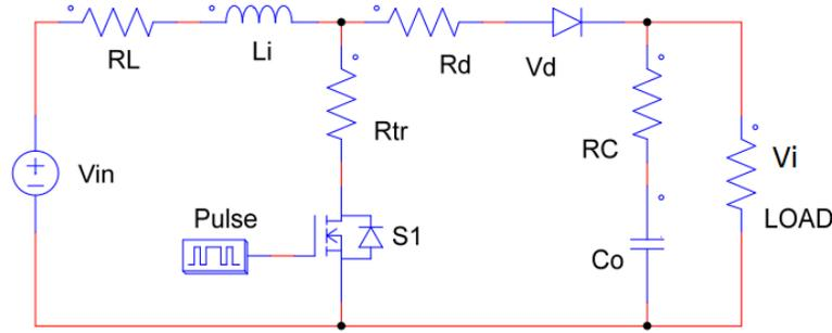
Figure 3. Non-ideal circuit model of a DC/DC boost converter (with only inner resistances)
