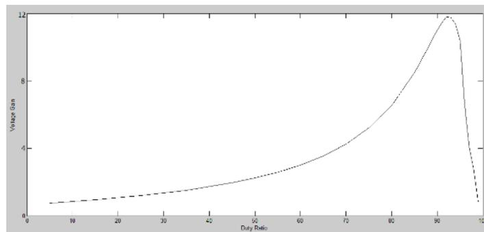
Figure 2. Voltage gain of a non-ideal DC/DC boost converter
