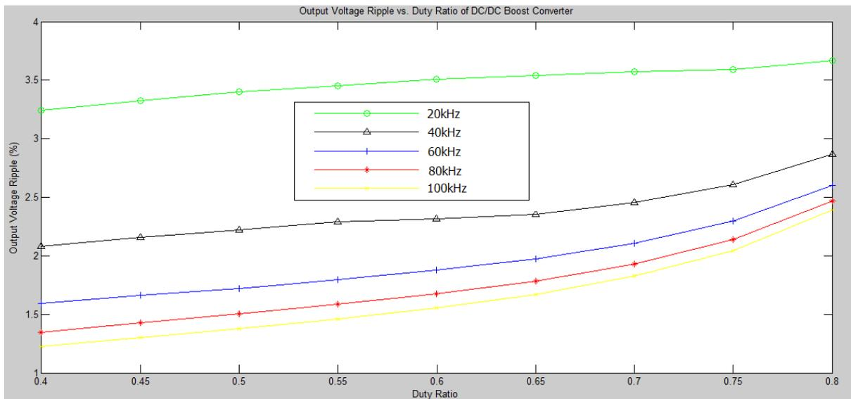
Figure 6. Voltage ripple vs. duty ratio graph of boost converter with respect to switching frequency
