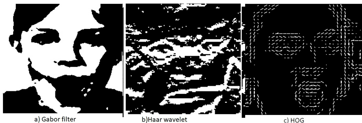
Figure 6. Segmentation result obtained from an image using Gabor filter (a), Haar wavelet (b), HOG (c) methods.
