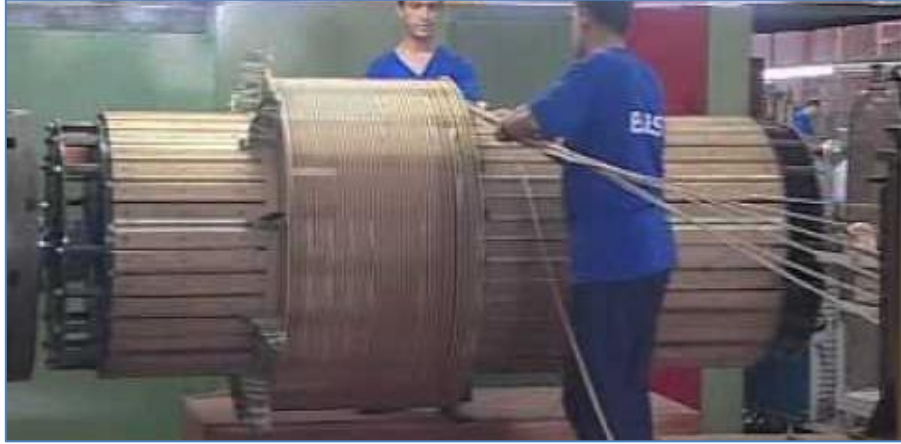
Figure 3. Transformer winding process
