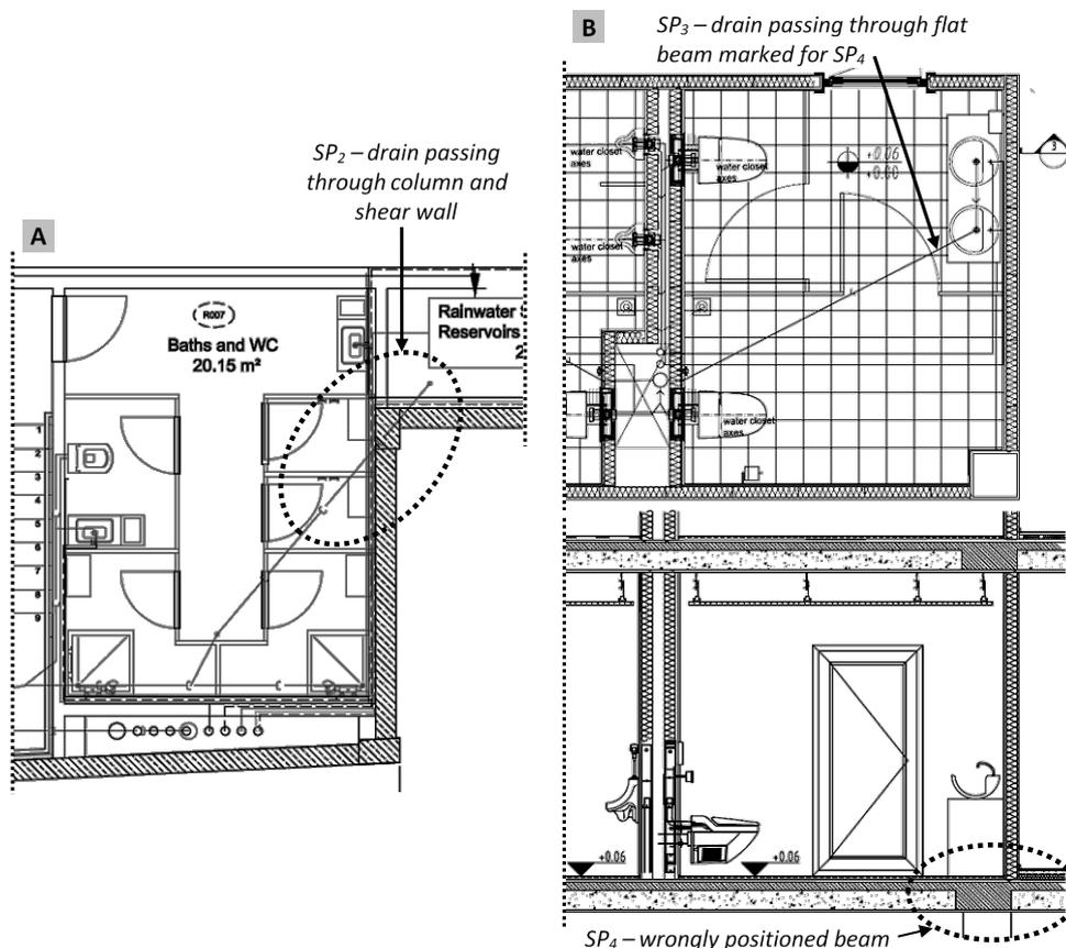
Figure 8: Examples of (A) SP<sub>2</sub> with hard clash, and (B) SP<sub>3</sub> and SP<sub>4</sub>.
