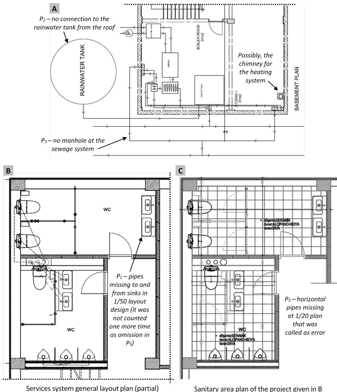
**Figure 3:** Examples of some plumbing system design deficiencies
