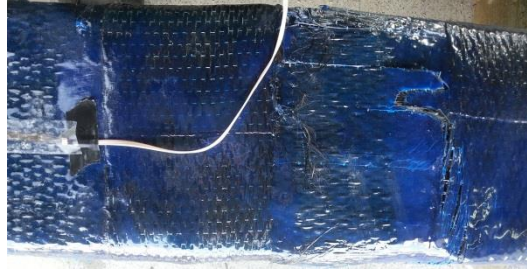
Figure 6. Rupture of CFRP on the tension face
