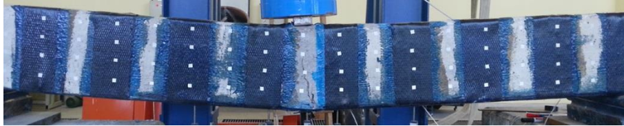
Figure 7. Crack pattern of DA4.5F3.0C10/10TII
