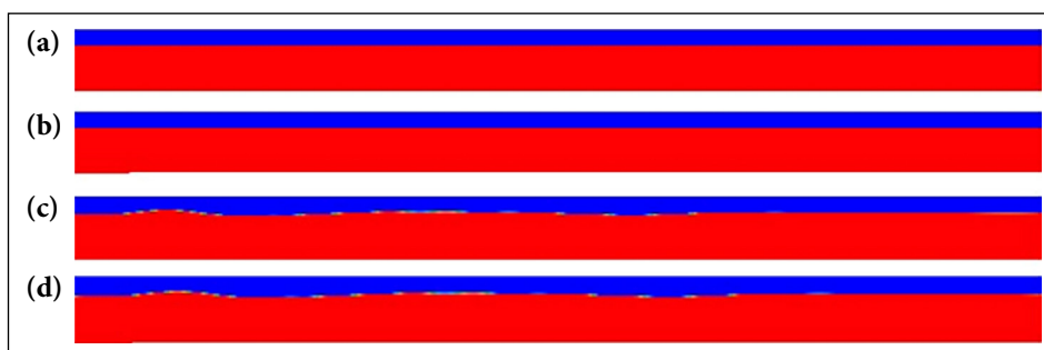
Figure 6. Elevation of the free surface at t=0 s for channels with (a) a flat bottom or (b) an inclined bottom and at t=900 s for channels with (c) a flat bottom or (d) an inclined bottom.
