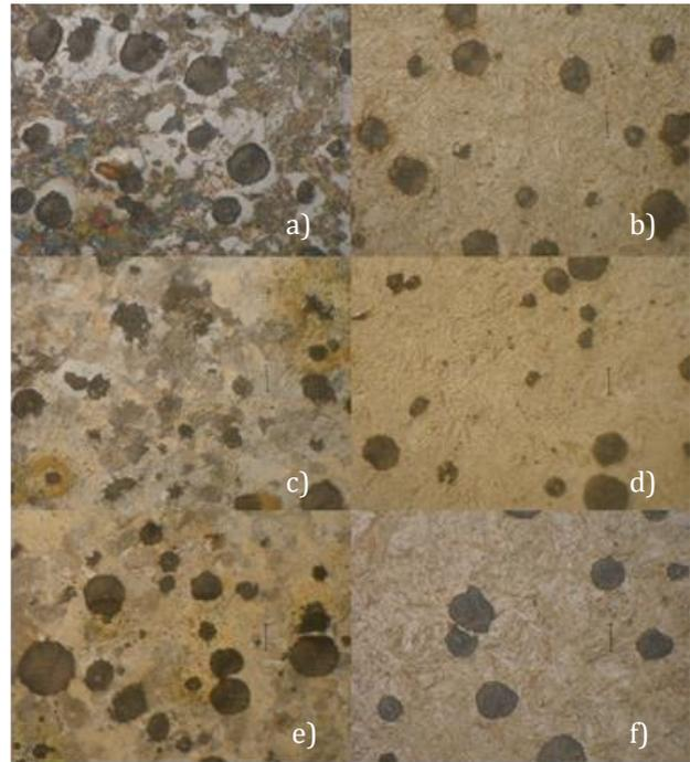
**Figure 3.** Metallographic photographs of 1000 °C annealed samples. (a and c and e air cooled samples, annealing time 1,2 and 4 hours respectively; b and d and f quenched samples annealing time 1,2 and 4 hours respectively)
