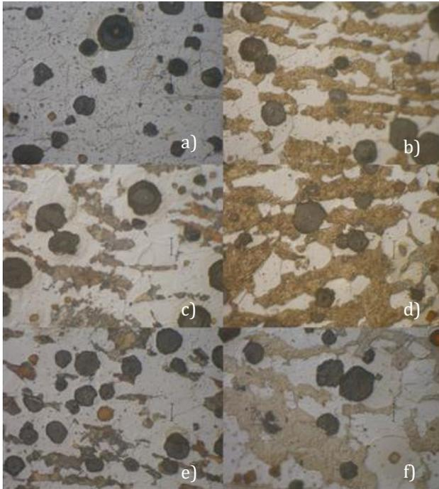
**Figure 2.** Metallographic photographs of 900 °C annealed samples. (a and c and e air cooled samples, annealing time 1, 2 and 4 hours respectively; b and d and f quenched samples annealing time 1, 2 and 4 hours respectively)
