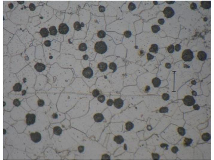
**Figure 1.** Original microstructure (Scale 20 micron)
