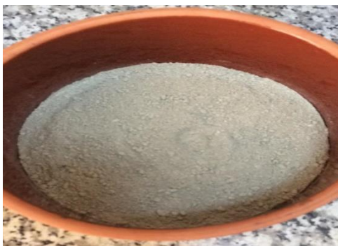
Figure 5. Collected PbSO_4 rich precipitate [The precipitate collected at conditions: 2 M sulfuric acid, 30 minutes leaching time, 25 °C temperature, 2/10 solid-to-liquid ratio (w/v), 125 rpm shaking rate].
