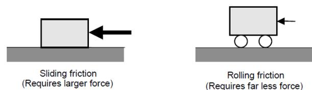
Fig. 3. Difference between sliding friction and rolling friction
