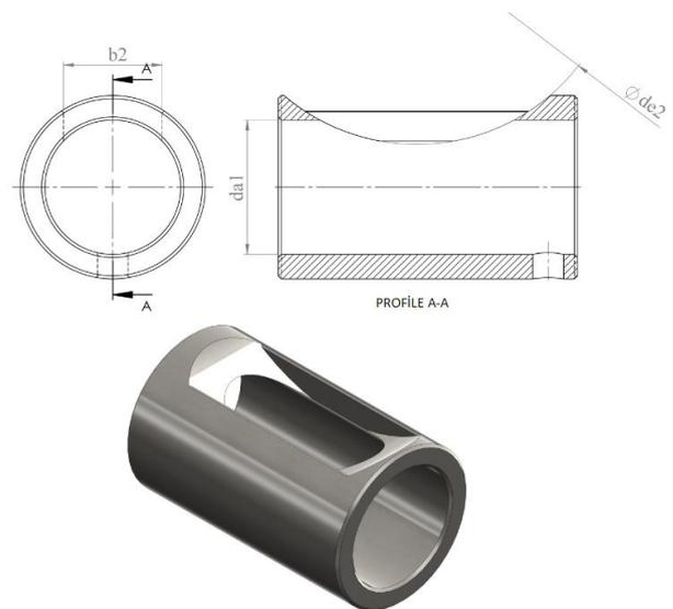
**Fig. 7.** Technical drawing of the guide sleeve
