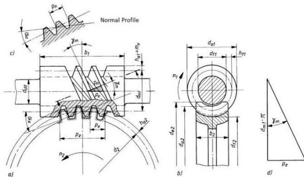
Fig. 1. Worm gear and worm wheel base
