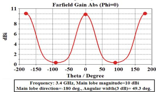
b) The radiation pattern characteristic for the resonance frequency of 3.4 GHz
