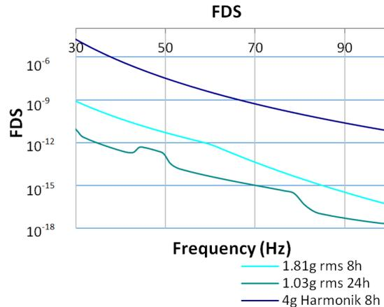
Figure 3. Comparison of FDS's of Random PSD G and 4g Harmonic Sweep
