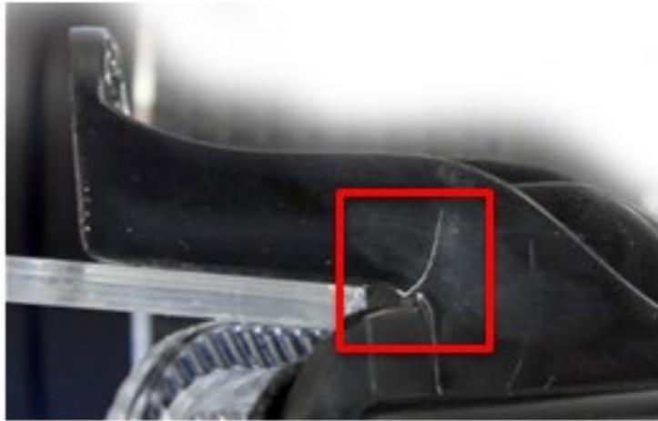
Figure 12. Crack Propagation on the forecasted critical area
