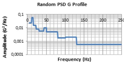
Figure 2. 24h duration Z axis, 5-250Hz, PSD G rms: 1.03g
