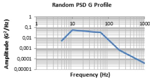
Figure 1. 8h duration Z axis, 5-1000Hz, PSD G rms: 1.81g
