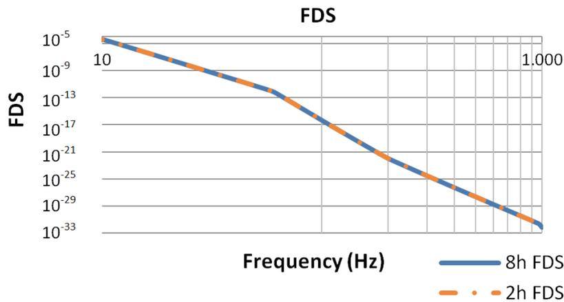
Figure 5. FDS curves for 8h duration PSD G and accelerated 2 h duration PSD G test
