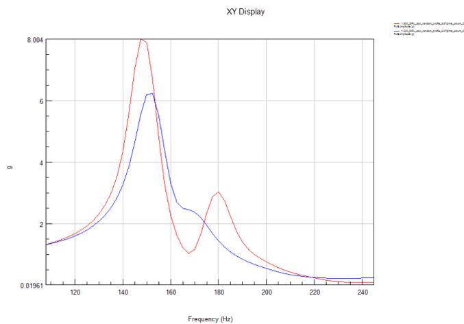
Figure 14. Acceleration Frequency Response Curves before and after crack
