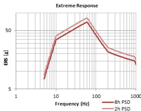
Figure 6. ERS curves for 8h duration PSD G and accelerated 2 h duration PSD G test
