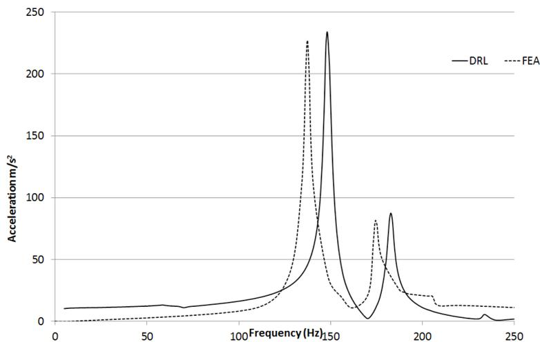
Figure 8. Comparison of resonance search result and FEA acceleration response result
