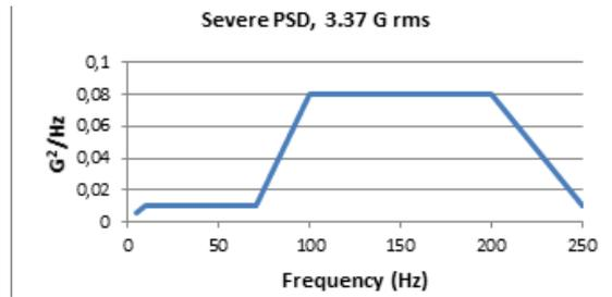
Figure 9. Severe PSD G
