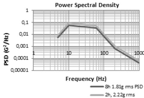
Figure 4. 8h PSD G and 2h PSD G
