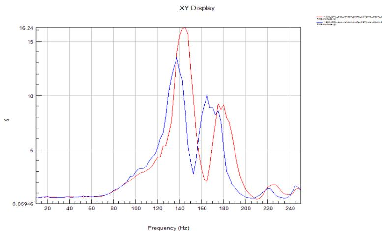
Figure 20. Acceleration Frequency Response Curves before and after crack
