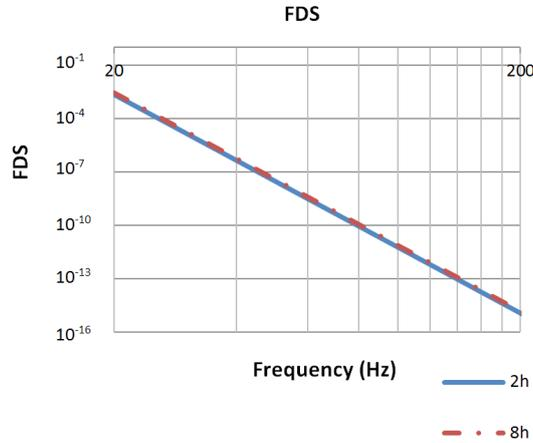
Figure 7. FDS for 8h constant g harmonic sweep test and accelerated 2h test
