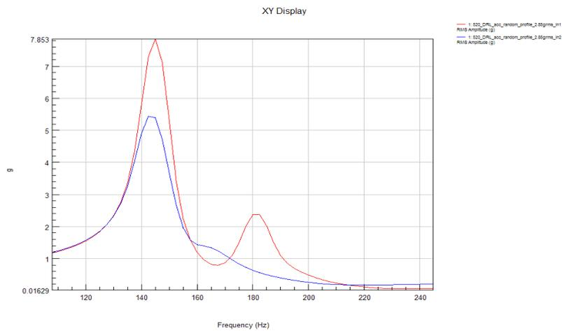
Figure 17. Acceleration Frequency Response Curves before and after crack
