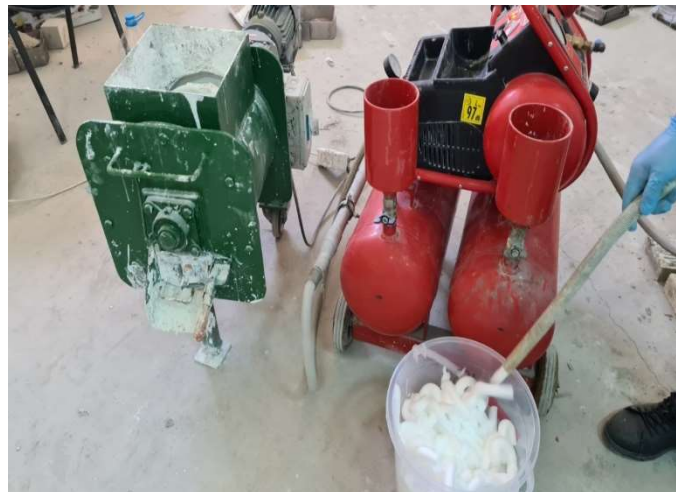
Figure 1. Foam production in a foam generator
