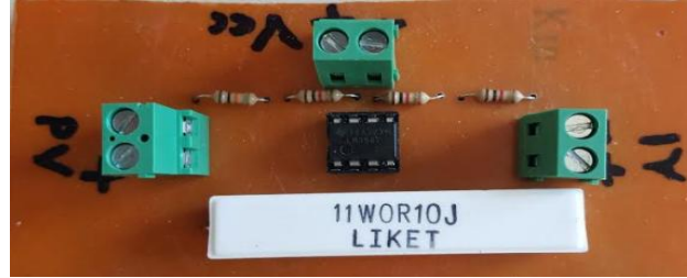
Figure 8. Printed circuit for current measurement (Top view).
