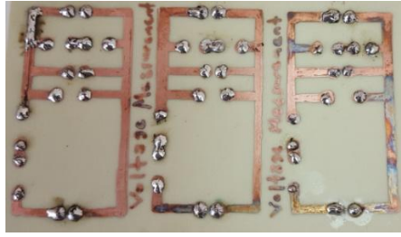
Figure 12. Printed circuit for voltage measurement (Bottom view).
