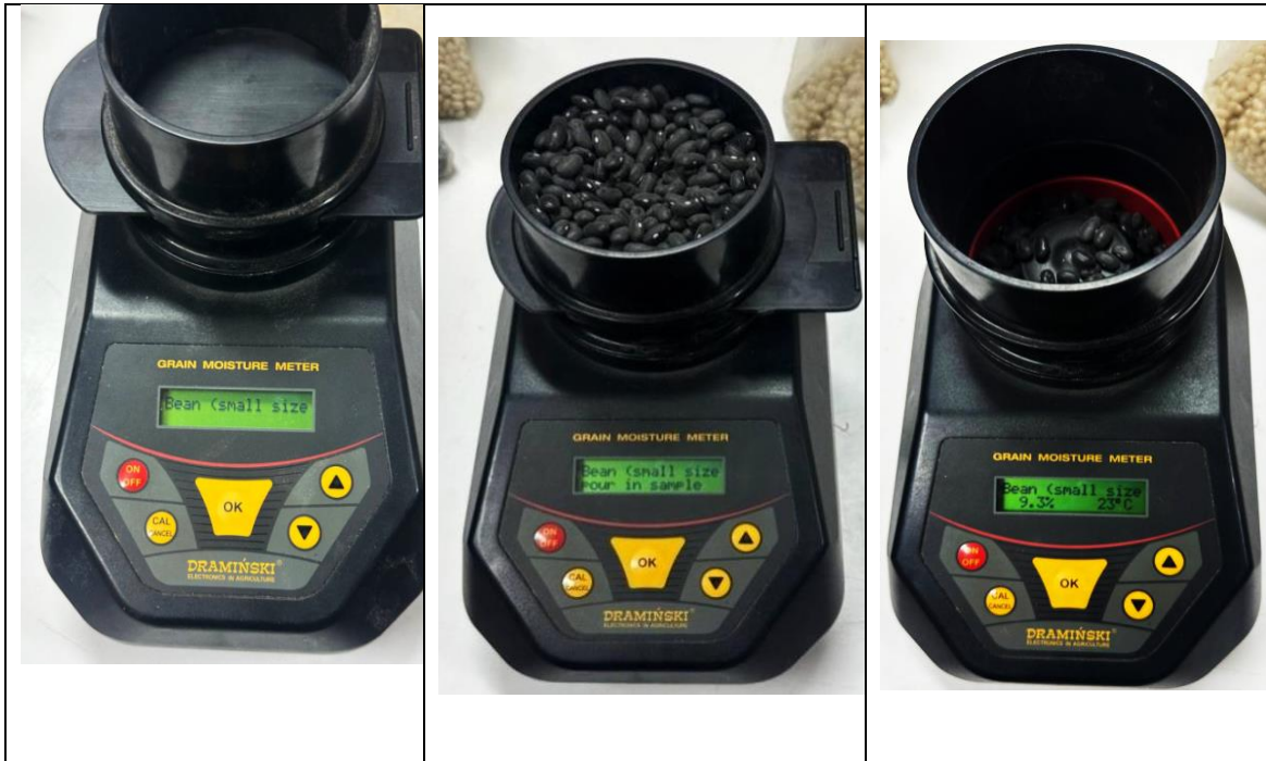
Figure 4. Grain moisture meter (Model: GMM mini DRAMINSKI, which is Origin Poland).
