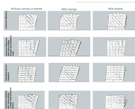
Figure 8. Failure types when the lateral load at the in-plane direction (modeled by the author via SketchUp 2017 and MsPhysics 1.0.3.)
