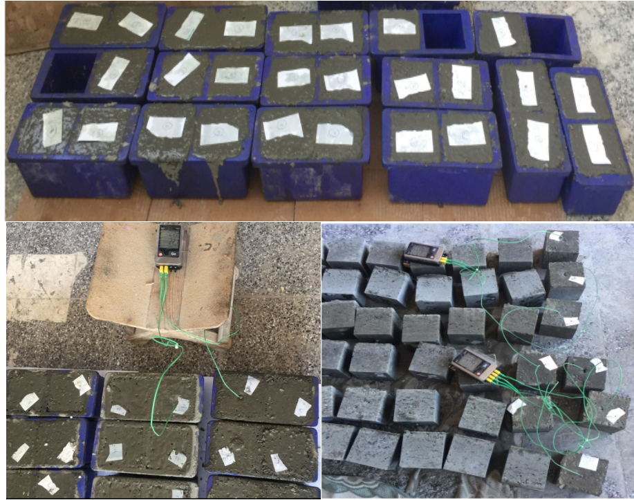
Figure 3. Placement of the temperature measuring device.
