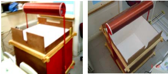
Figure 2. Two different aspects of the magnetic field source.
