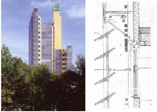
Şekil 19. Berlin Debis Building, Renzo Piano, Christoph Kohlbecker, 1997, Berlin, (Çift Cidarlı Cephe Uygulaması) (Application of Double Walled) (35)
